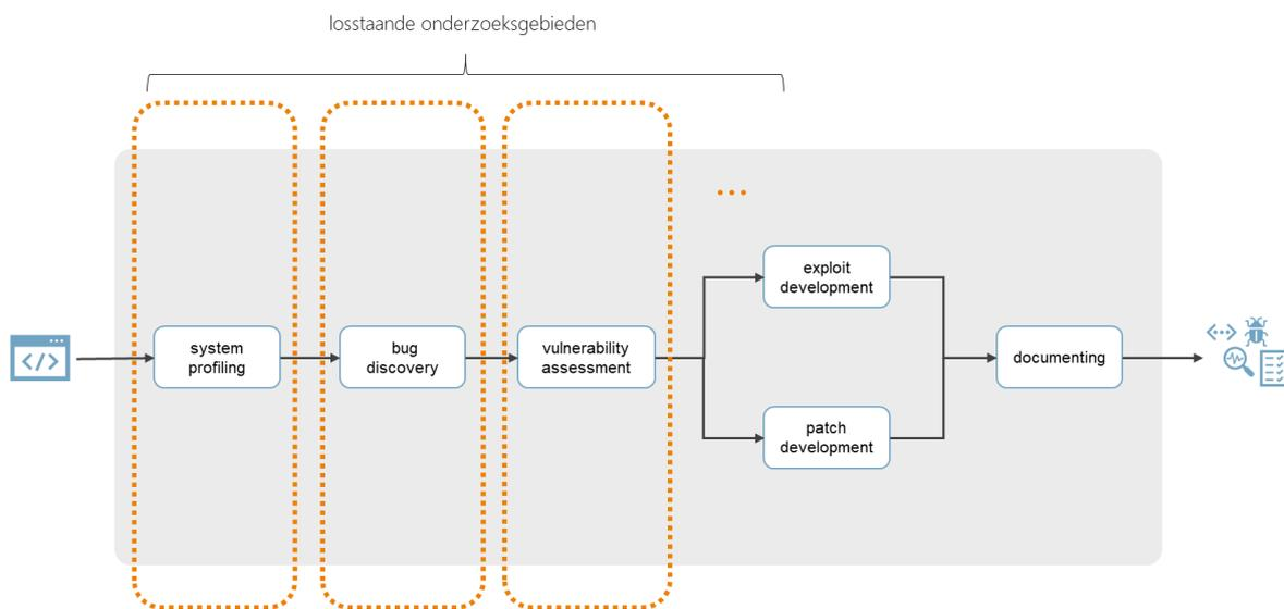
Figure 4: The various process steps within AVR.
